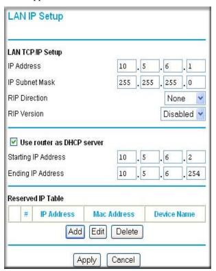
Figure 6-8: LAN IP Setup menu
